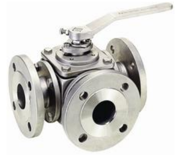
DJV-9308 (Full Bore) Trunnion Ball Design, Multiple Packings, One-Piece Ball & Stem, Square Stem, 360° Rotation
