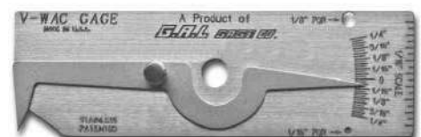
V-WAC #5 Checks undercut, crown height, porosity, pits, in stainless steel, metric or inch
